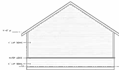
2 | Rear Elevation EXISTING
