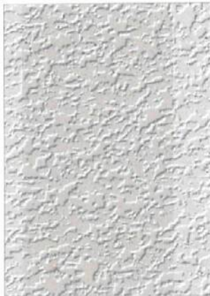
ST-1 (3 COAT STUCCO) PAINTED - SW 6385 DOVER WHITE
