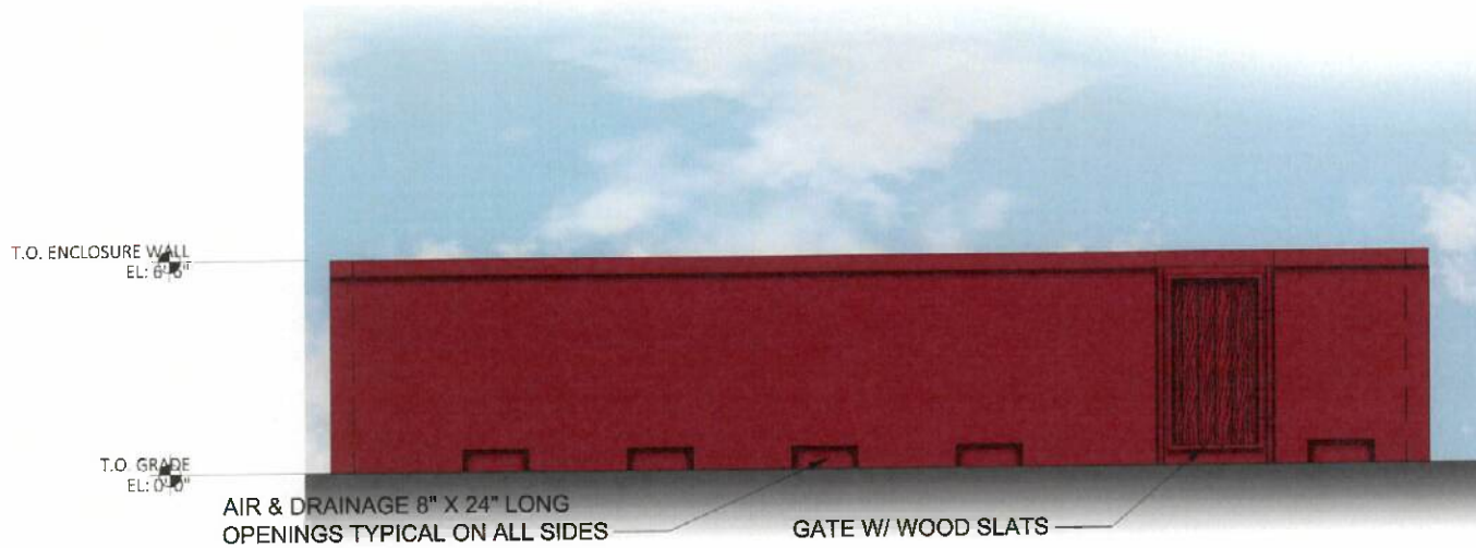
1 PROPANE ENCLOSURE FRONT ELEVATION SCALE: 1/4" = 1'-0"
