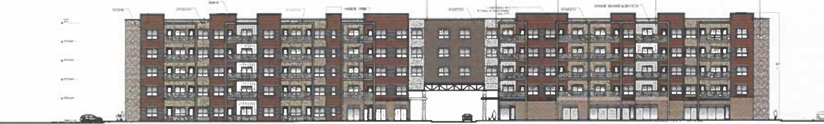
EAST ELEVATION - BUILDING C 1/8" = 1'-0"
