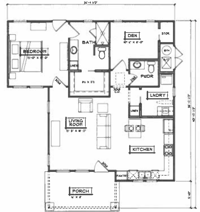
FLOOR PLAN SCALE: 1/8" = 1'-0" || PAPER: 1/4" = 1'-0" || 34" X 34" PAPER LIVING AREA - 1042 S.F. 1 PORCH AREA - 81 S.F.
