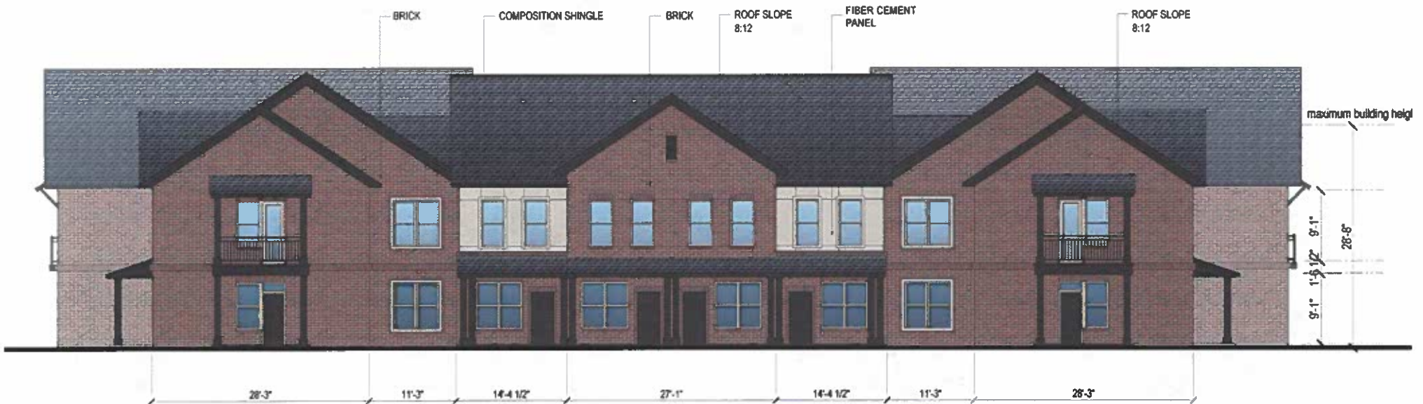
BUILDING I - REAR ELEVATION
