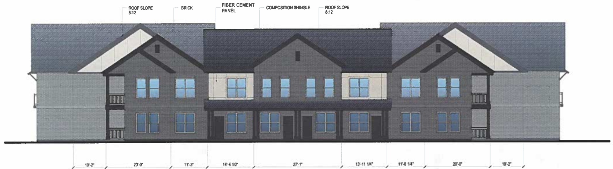
BUILDING II-REAR ELEVATION
