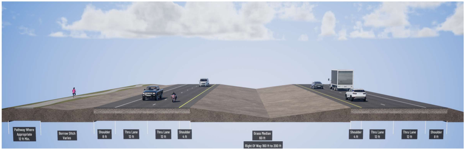
FIGURE 6: EXAMPLE EXPRESSWAY CROSS-SECTION
