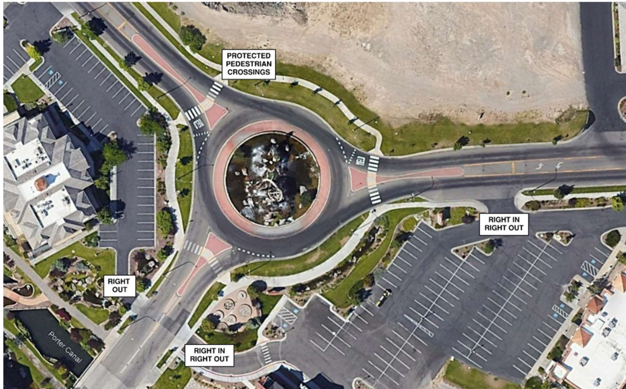
FIGURE 5. EXAMPLE OF ACCESS MANAGEMENT NEAR ROUNDABOUTS
