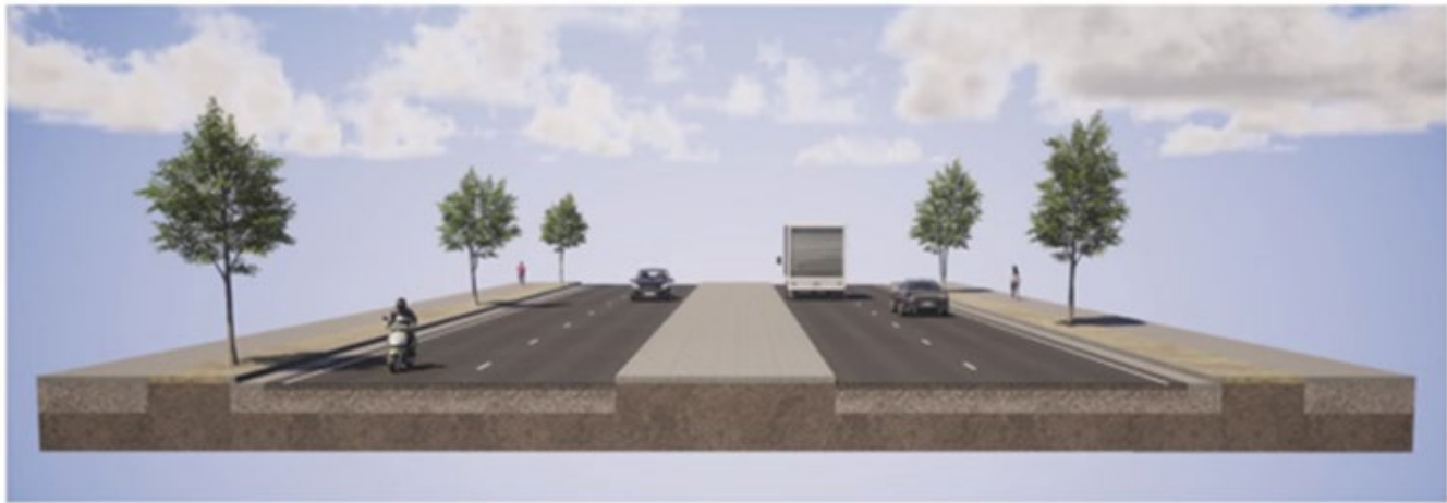
FIGURE 8: STRATEGIC ARTERIAL POTENTIAL CROSS SECTION
