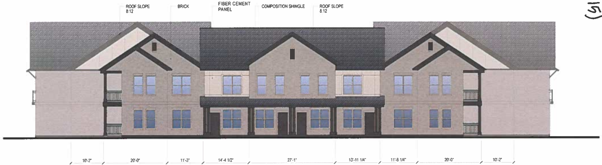
BUILDING II-REAR ELEVATION
