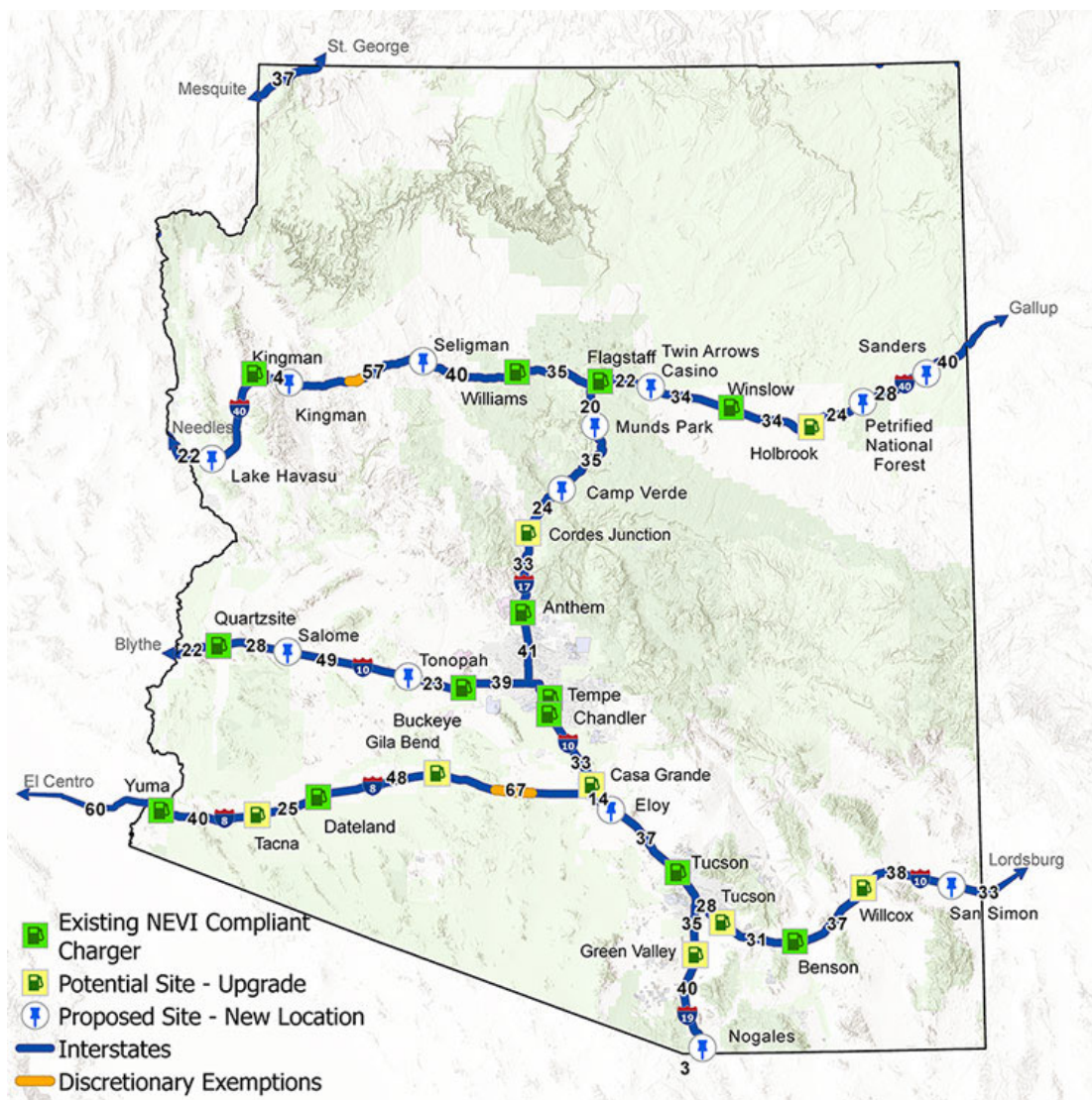
Figure 7: ADOT Phase I EV Charging Locations
