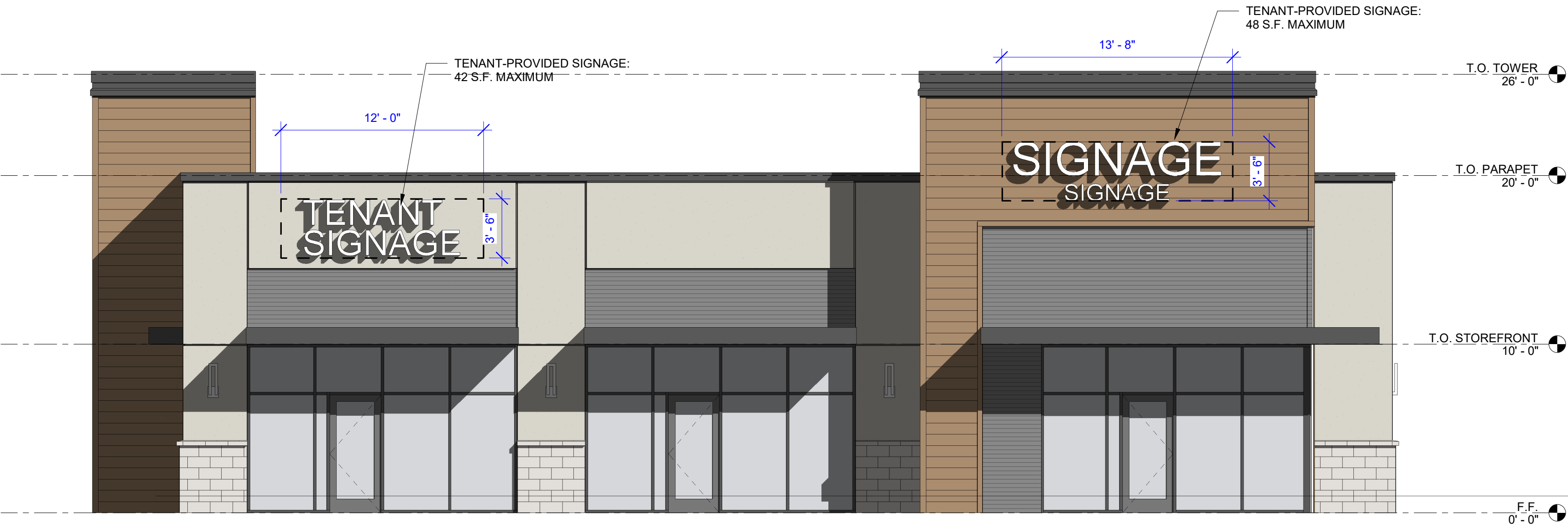
WEST (FRONT) ELEVATION - SIGNAGE
