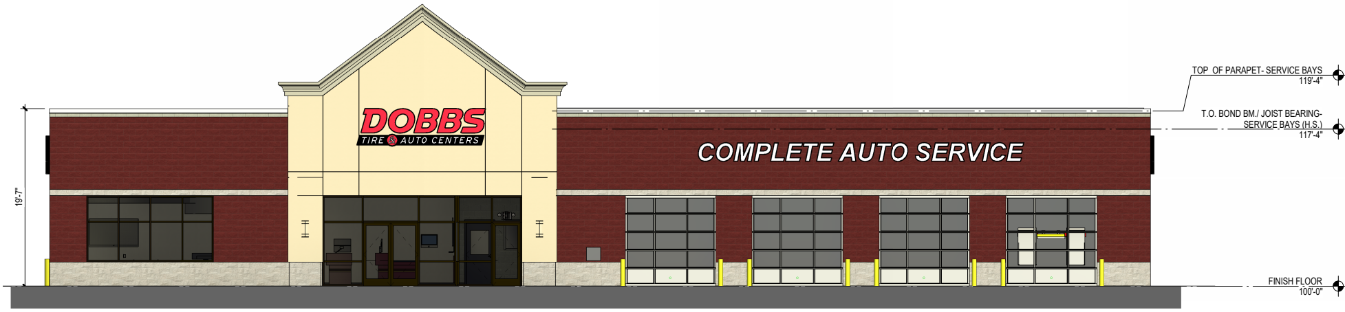
FRONT FIELD: SPLIT-FACE CMU - ACCENT SPLIT-FACE CMU - ACCENT SMOOTH FACE CMU - EIFS FRONT ENTRY
