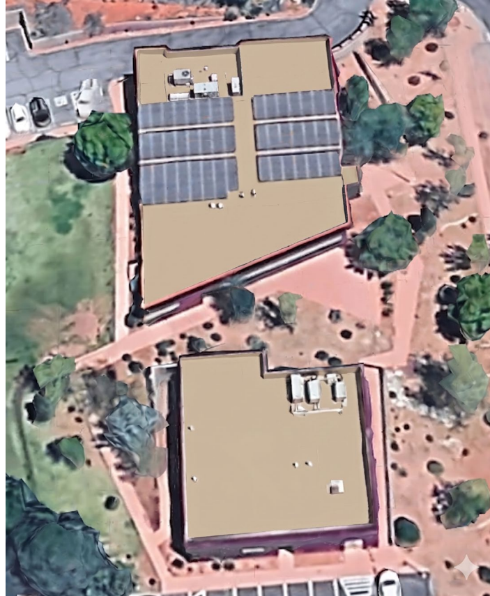
Figure 12 Proposed Cool Roof Model in the Brewer Road Buildings
