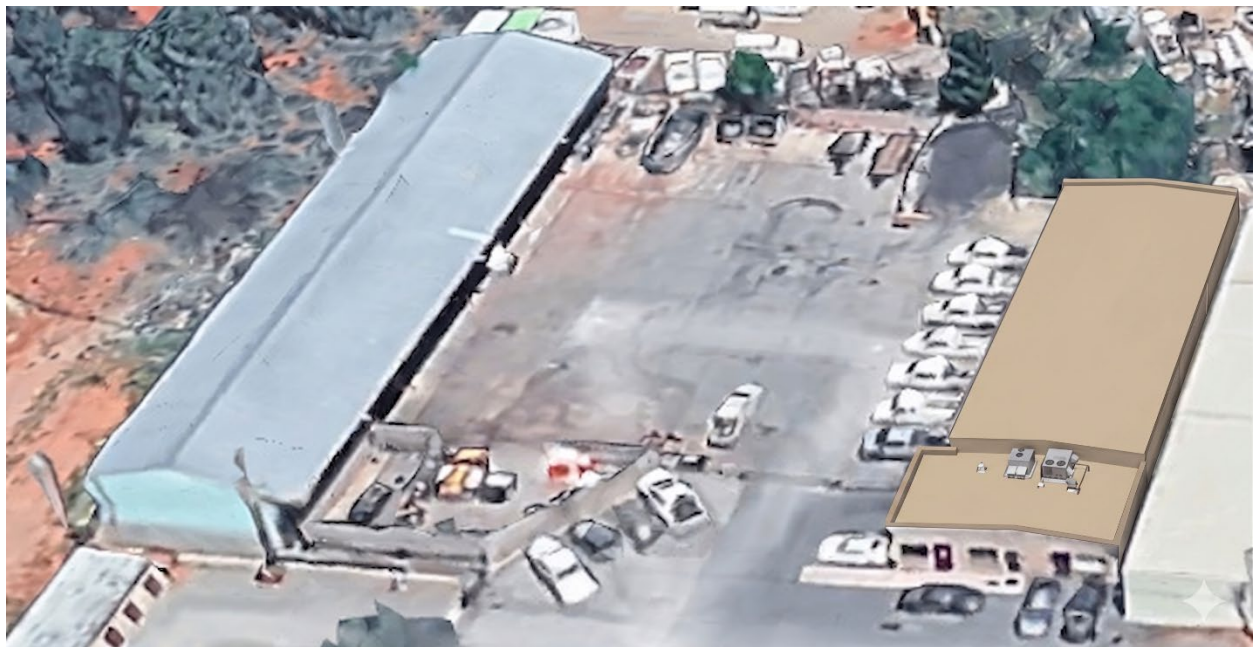
Figure 15 Existing Metal Roof with White Coating
