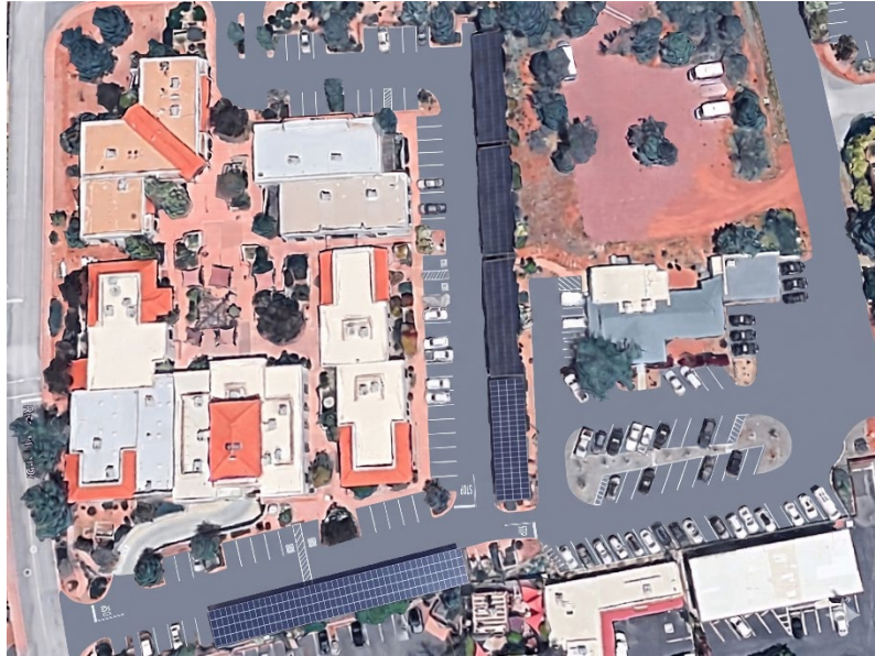
Figure 22 Proposed Gray Cool Pavement Layout in 102 Road Runner Drive
