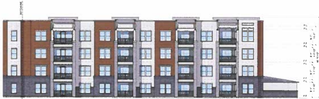
01 BUILDING 'C' REAR ELEVATION SCALE: 1/8" = 1'-0" 1 REQUIRED @ BUILDING 3
