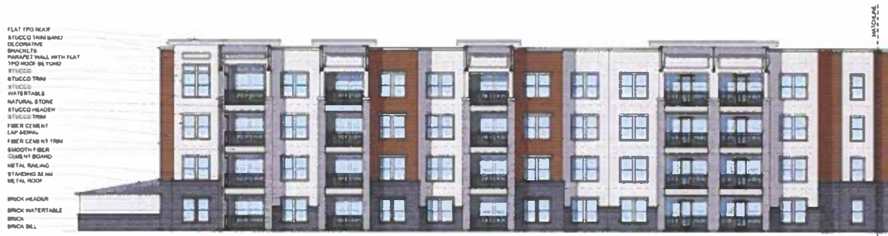
02 BUILDING 'C' REAR ELEVATION SCALE: 1/8" = 1'-0" 1 REQUIRED @ BUILDING 3
