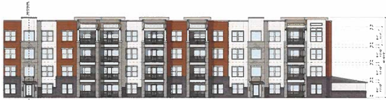
01 BUILDING 'C' FRONT ELEVATION SCALE: 1/8" = 1'-0" 1 REQUIRED @ BUILDING 3
