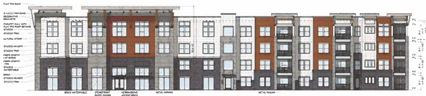
01 BUILDING 'A' FRONT ELEVATION SCALE: 1/8" = 1'-0" 1 REQUIRED @ BUILDING 1
