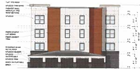
03 BUILDING 'C' RIGHT ELEVATION SCALE: 1/8" = 1'-0" 1 REQUIRED @ BUILDING 3
