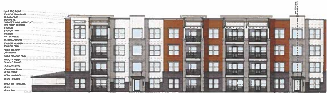
02 BUILDING 'C' FRONT ELEVATION SCALE: 1/8" = 1'-0" 1 REQUIRED @ BUILDING 3
