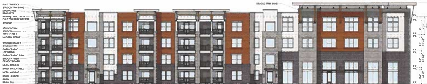
01 BUILDING 'A' LEFT ELEVATION SCALE: 1/8" = 1'-0" 1 REQUIRED @ BUILDING 1
